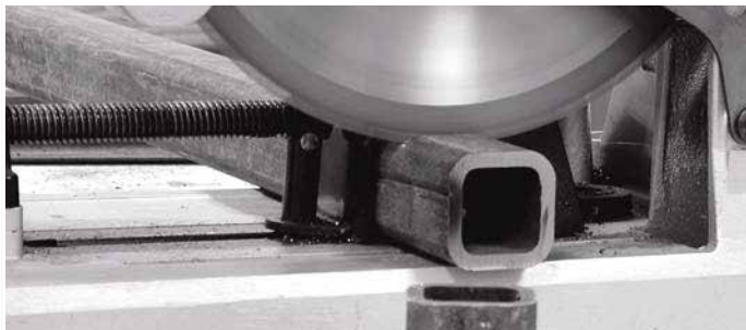
Carbide-Tipped Blades make Virtually Spark-Free Cuts
